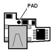
Finally solder 1 wire from the **PAD** of the USB charger PCB to the **battery clip** inside the **lower case**. Then solder a 2nd wire from **PAD** to **BT+**.
